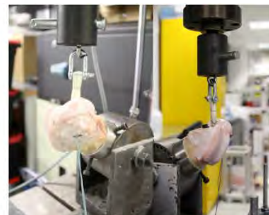
Figure 4. Graft-Tunnel stability under cyclic loading Biomechanical Testing
