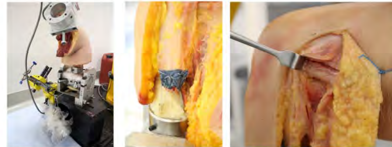
Figure 1. Iliotibial tract loaded with 30 N within a 6 degrees of freedom robotic testing system
